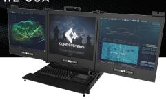
The triple 19" display has a native pixel resolution of 1280 x 1024 and is built with antireflective glass. The triple LED display features zero defects out of the box, a sealed full travel keyboard and an integrated touchpad or trackball pointing device. The SWaP-Optimized MLD3K utilizes 3U height and is 20 inches deep. With an industryleading rugged design, this triple 19" panel mount LCD is perfect for missions of all kind.
