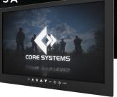
The SWaP-Optimized MPN19W utilizes 8U height and is less than 3 inches deep. With an industry-leading rugged design, this 19" rugged display is perfect for missions of all kind. The MP19W can be modified to your specifications and we specialize in quick turnarounds.
