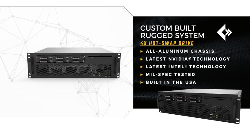
Built with ultra-sturdy all-aluminum chassis, this rugged computer features four shock-mounted hot-swap drives and supports the latest Intel® Quad and Hexa-Core CPUs while providing six full-height PCIe slots on the rear of the chassis. The rugged M318S includes the latest single-stack NVIDIA® Tesla® GPU Card which provides our customers with high-performance data analytics and scientific computing abilities.
