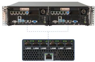
Each node includes 7x independently operating 1GB ports allowing users to set up seperate, individual networks
